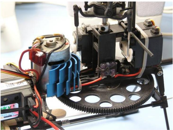
In the picture above you can see the location of the two fuses. Use a 7.5 Amp fuse on the main motor. Trim the fuse terminals and bend them into position. Then solder the fuse directly to the terminal on the side of the motor and solder your wire to the other terminal of the fuse (as shown).
