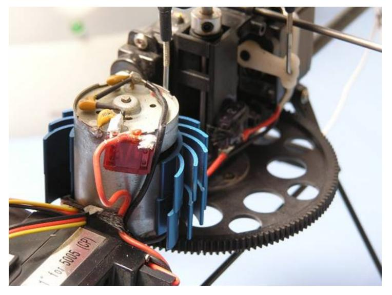
Here is a view from the front. Again- make sure neither of the fuse contacts touches the metal case of the motor. If it touches the motor can then you will probably damage your speed controller (4 In 1 Controller).
