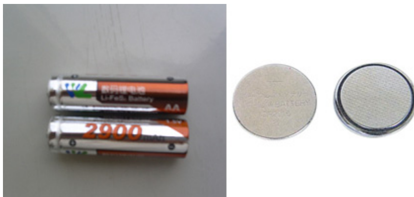
Figure 1 - Example of Lithium Metal Batteries
