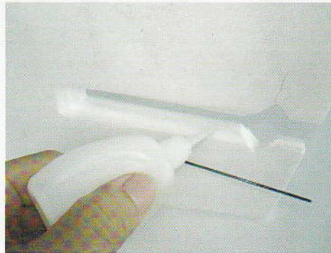
18. THE GLUE SPREAD ON THE FIXED HOLE OF HORIZONTAL TAIL 18: 将胶水涂刷到平尾固定槽位中
