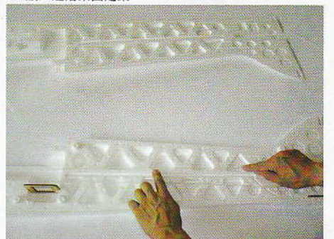
10. THE PP PIPE GULE TO FUSELAGE 10: 放上天线导管
