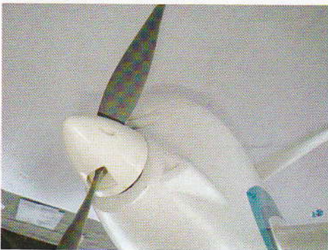
37. ASSEMBLE PROPELLER AND SPINNER
