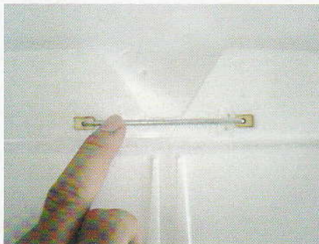
17. THE WIRE IS GLUE TO THE ELEVATOR 17: 用胶水装入升降舵钢丝
