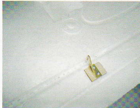
30. ASSEMBLE WINGS OF FORTIFIED WOOD AND HORN 30: 副翼装上加强木片和舵角
