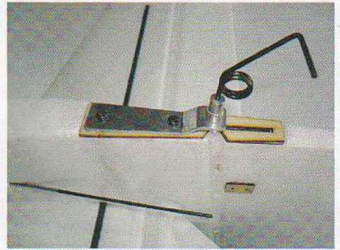
25. ASSEMBLE THE WIRE OF TAIL WHEEL 25: 装上尾轮钢丝
