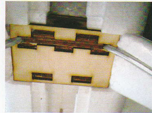
41. THRUST THE FIXED WOOD INTO LANDING GEAR MOUNT
