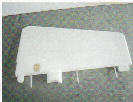
21. THE HINGE IS GULE TO THE HOLE OF VERTICAL TAIL 21: 将铰链插上方向舵中
