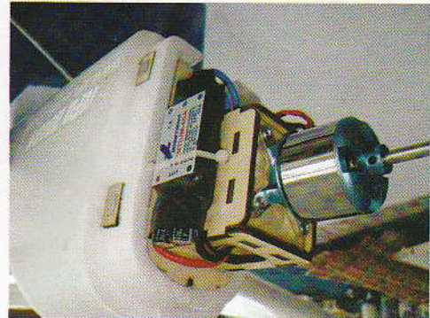
35. ASSEMBLE MOTOR AND ESC, ATTENTION MOTOR RIGHTWARD 1.2° AND DOWNWARD 1°
