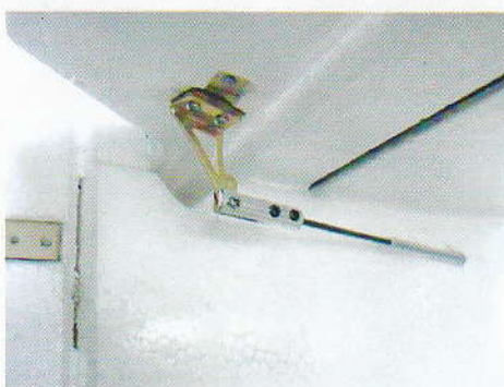
33. ASSEMBLE ELEVATOR SERVO CLEVIS, MOBILE ANGLE IS 20MM 33: 装上升降舵夹头, 上下活动角度是20MM
