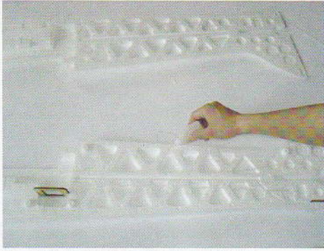
11. THE GLUE SPREAD ON FUSELAGE 11: 机身加上胶水
