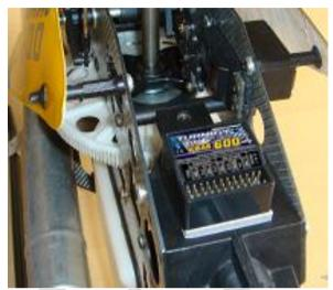
Turnigy® V-Bar 600 can also run perpendicular to the helicopter's nose
