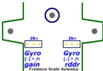
Fig. 1: Plug gyro leads into Arizona Regulator so that the conductors are (-), (+), and (SIGNAL) as viewed from left to right.
